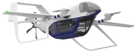
Fig. 11 TF-2 Lift + Push (Lavars, 2018)
