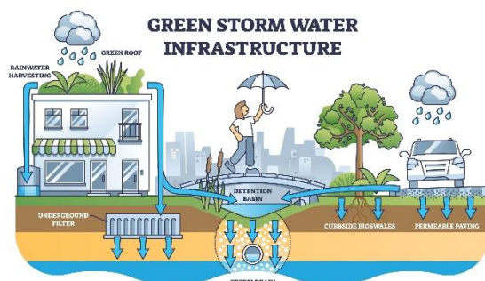
Fig. 1. A visual overview of green stormwater infrastructure, a sustainable approach to managing urban stormwater runoff.
